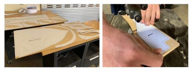
There are plenty of materials which could be used to make panels, but we considered using either MDF or plywood as they are cheap and easily cuttable. We ended up deciding to use MDF for the purpose of cleaner manufacturing as it doesn't splinter like plywood.
